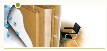
The plaster base board is designed specifically for use in timber frame construction, in respect of format, rigidity and hydrophobic property. It may therefore be mounted directly on the wall studs, creating a perfect and stable substrate for plastering.
