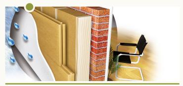
Thermal bridges are largely avoided. Thicknesses up to 160 mm assure outstanding thermal protection in a single work step.
