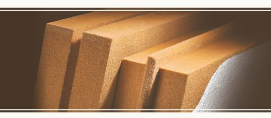
The homogeneous plaster base board for composite thermal insulation systems (CTIS) in timber frame constructions, CTIS EnergiePlus comfort, manufactured using an innovative dry process. Fitted with tongue and groove, plaster base boards are mounted full surface directly onto the timber studs.
